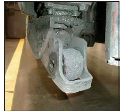
Deteriorated wheels, excessive surface wear and spalled joints are telltale signs of an owner who is not "floor conscious."
