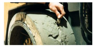
Deteriorated joints can cause extensive damage to material handling vehicles, resulting in reduced operational productivity and excessive MHV maintenance and repair
