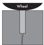
1. Semi-rigids provide edge support when they directly abut the side of the joint and the top joint edge.
