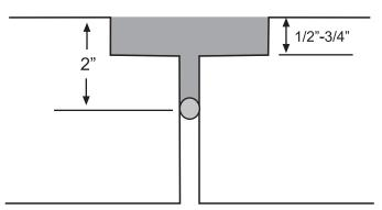
**Step 5** - After MM-80 cures into solid (approx. 6-8 hours at 70F) grind off overfill until mortar is flush with floor surface using ZEC pad or similar grinding disc.
