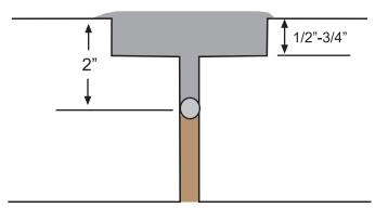
**Step 4** - Slightly overfill newly created channel with sand modified MM-80 Epoxy Joint Filler. To make mortar, mix MM-80 neat for 2-3 minutes then add clean, dry silica sand gradually 1/2 gallon at a time up to a maximum of 2 parts silica to 1 part epoxy.
