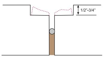
**Step 3** - Remove any high spots between new saw cut edges and existing joint with chisel or similar tool to establish shelf. Vacuum clean. Place backer rod in compression at 2" deep or depth of saw cut if material loss is a concern.
