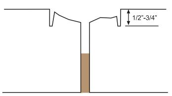
**Step 2 -** Clean original joint to depth of original saw cut or 2" for thru-slab joint or to original saw cut joint depth. (Thru-slab joint shown).
