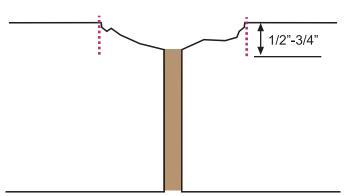
**Step 1** - Saw cut straight down 1/2" (minimum) to 3/4" (preferred) deep behind spalled edges using concrete saw (preferably dustless) equipped with diamond cutting blade.
