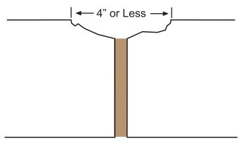
**Existing Condition** - severe joint spalling on both sides of the joint, up to 4" in width
