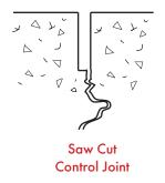
We stated earlier that a rule of thumb is that conventional concrete may shrink at a rate of 1/8" in 20'. Thus, for heavy duty floors, the use of smooth dowels should be considered to ensure positive load transfer.
