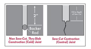
In construction (formed) joints that are not saw-cut, **Edge-Pro 80** should be installed at a minimum 2" depth. **DO NOT USE COMPRESSIBLE BACKER ROD IN STANDARD SAW-CUT CONTRACTION/CONTROL JOINTS!** Rod may be used
