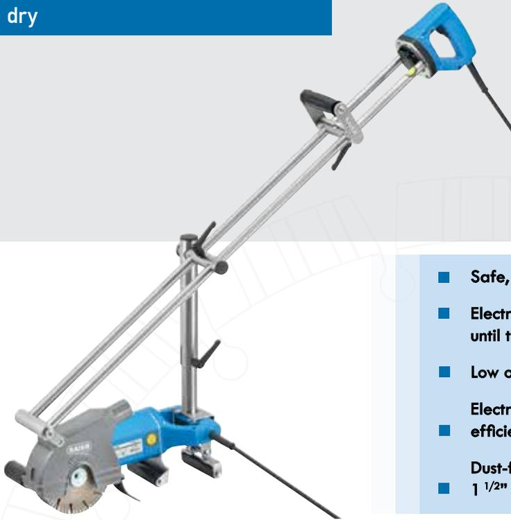
Diamond floor channel cutter with 11 diamond cutting blades for bridgeless milling up to 2" wide and 1.8" deep
