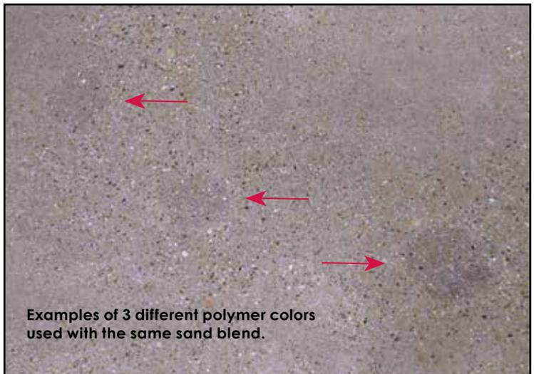
Examples of 3 different polymer colors used with the same sand blend.
