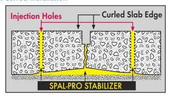
Corrective procedures may vary due to conditions (severity of curl, degree of deflection, joint edge spalling, etc.). Contact Metzger/McGuire for assistance in determining best methods for slab stabilization.
