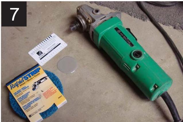
Rapid Refloor will harden quickly (within minutes). Wait 30 minutes or more, then grind off overfill using a grinder and medium grit finishing pad such as the Norton Rapid Strip disc. Grinding can be done next day if desired.
