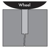
2. Semi-rigids provide edge support when they directly abut the side of the joint and the top joint edge.
